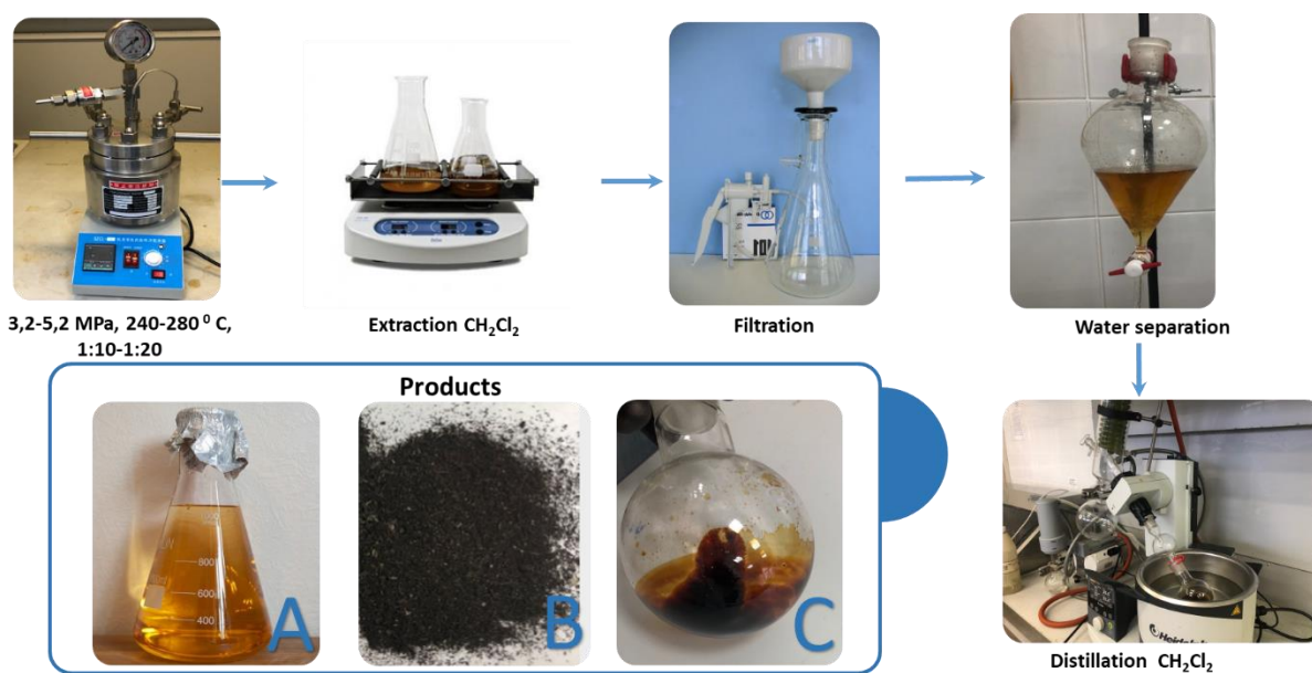
Figure 1. Scheme of the process of hydrothermal liquefaction of excess activated sludge: A – aqueous phase, B – coal residue, C – bio-oil.
