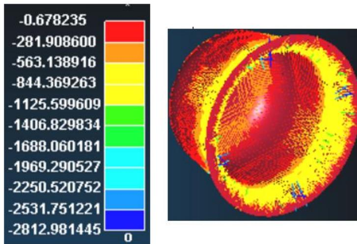
Fig. 5. Stress distribution along the Z-axis
