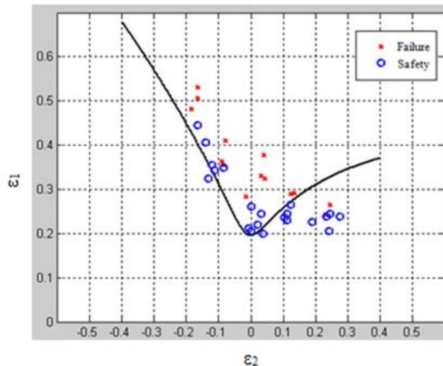
Fig. 3. The forming limit curve
