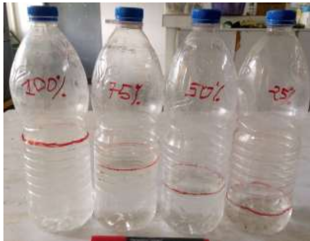
Figure 3. Transparent bottles containing 800, 600, 400, and 200 ml of water corresponding respectively to 100, 75, 50 and 25% of water regime (WR).
