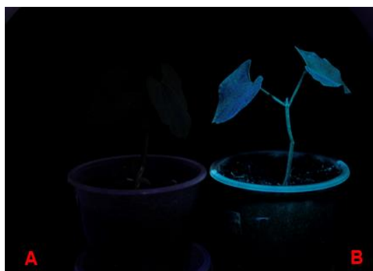
Figure 2 - Application quality methodology on bean leaf ( Phaseolus vulgaris ) seen with ultraviolet light. A. Water application. B. Product Application.
