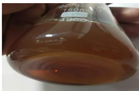
Figure 1: Aloe vera based synthesized nanoparticles: A brownish orange solution was formed which confirms the result of nanoparticles is formed
