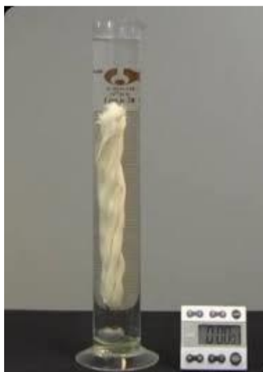
Figure 3. Wetting efficiency by Draves test
