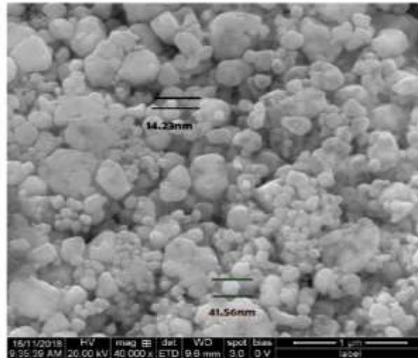
**Figure 4 High resolution scanning electron microscopic (SEM) image of silver nanoparticles (AgNPs). Polydispersed (Cluster) AgNPs ranged between 14.23 to 41.56nm.**
