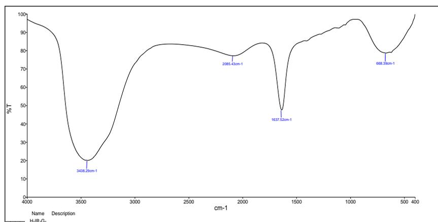
**Figure 3 FTIR analysis of silver nanoparticles synthesized by treating 1mM aqueous  $\text{AgNO}_3$  solution with *Sansevieria roxburghiana* leaf extract.**
