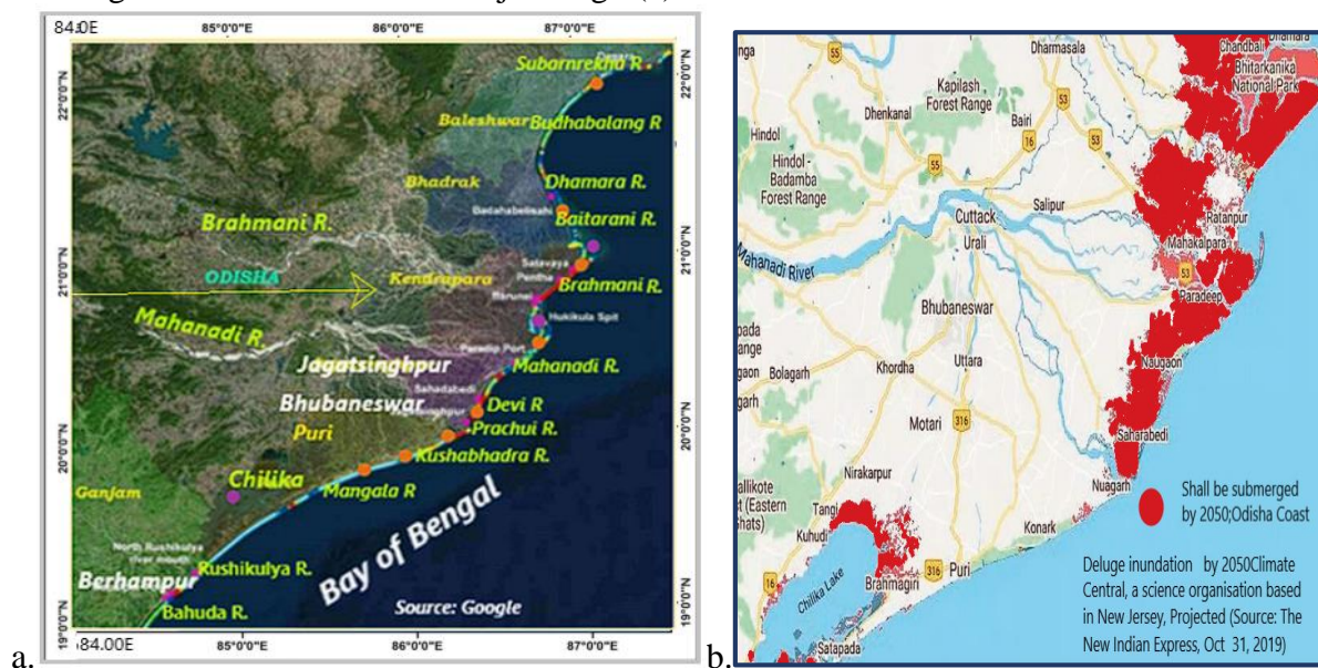
Fig 2 (a): The coastal map with the drainage system of Odisha with Chilika Lagoon (b) the projected inundation map of Odisha's coast by 2050
