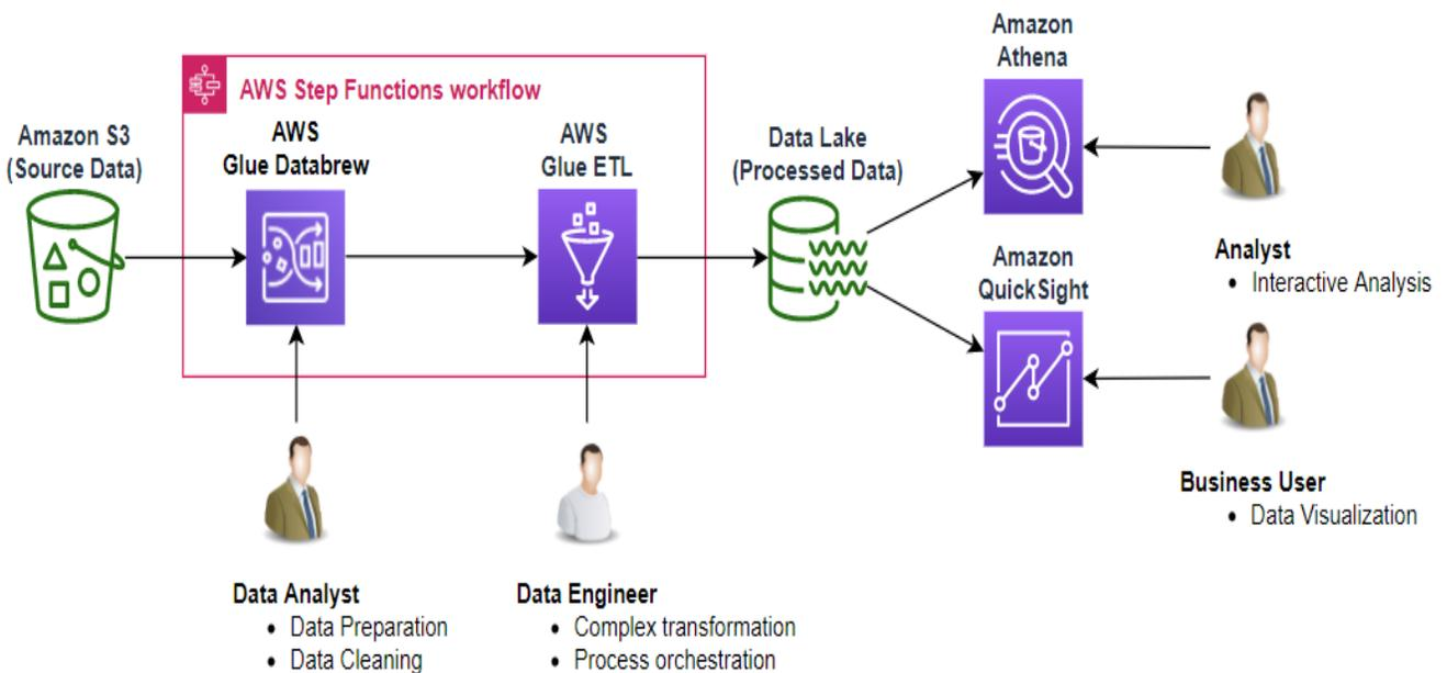
Fig.2. AWS Step Functions Workflow
