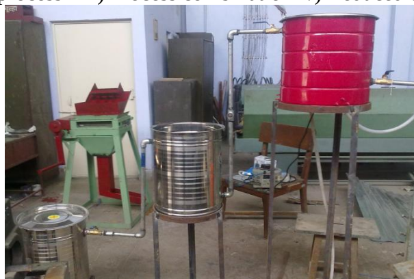
Fig 2: Continuous type sugarcane juice clarifier
