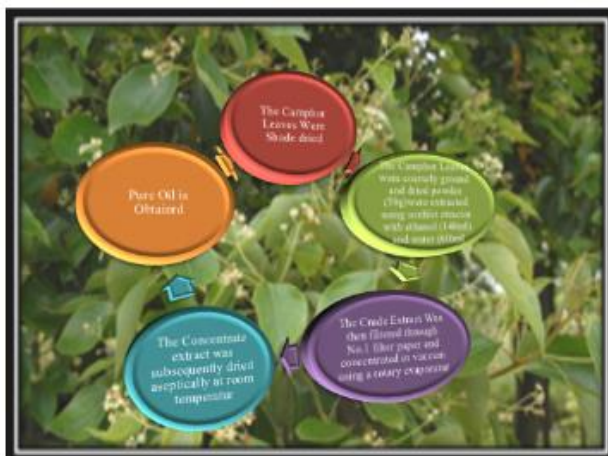
FIG. NO 4- EXTRACTION OF NATURAL OIL BY SOXHLETION
