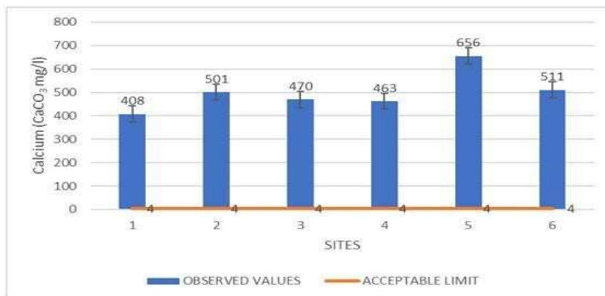
Figure 8: Concentration of CaCO 3 (mg/l) in soil and slurry samples collected from different sites
