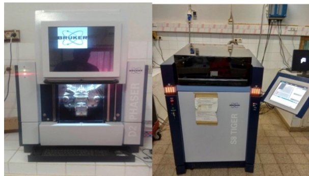
Figure 3: (From left to right) D-2 diffractometer and S8-Tiger spectrometer from Bruker (Boullé, 2017)
